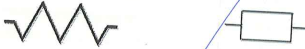
Fig 3.2 Symbols used to represent a resistor based on IEEE and IEC standards.
